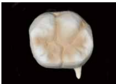
Fig13 Shading zirconia with colouring agent before strengthening
