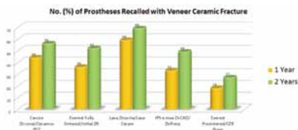
Fig8 Veneer ceramic fracture rate of 3-unit bridge with hand-layering technique and pressed-on technique. All of the products were fabricated with hand-layering technique except Zirpress and CZR, which was made by Press-on technique. (data from Christensen et al., 2010)
