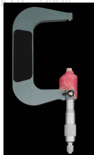
Figure 2. Fabrication of acrylic artificial gum (Hygenic Repair Acrylic (Coltene Whaledent) on the frame of a micrometer
