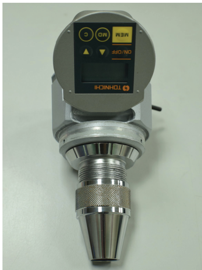
Figure 1. Digital torque gauge (TOHNICHI BTGE50CN-G) (Tokyo, Japan, Tohnichi Mfg.)
