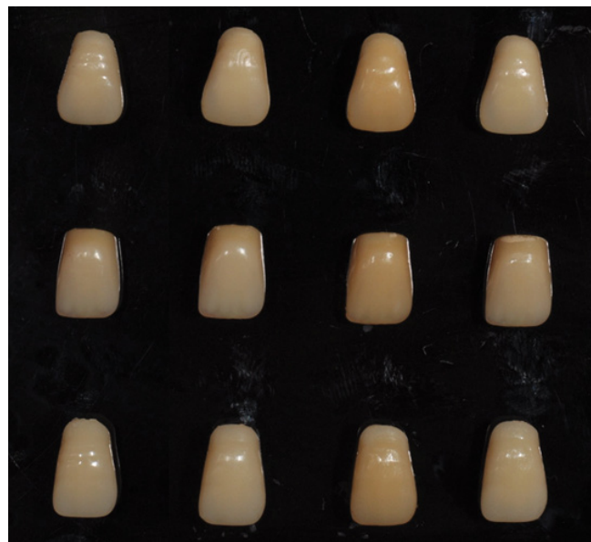
Figure 3. The groups from top to bottom are as follows: EFUCERR-A(E), SR Vivodent PE(V), Fx(F). The groups from right to left are as follows: No surface treatment (Control), grinding and conventional polishing (G+P), grinding and palaseal (G+Ps) coating, grinding and Optiglaze (G+Og) coating.
