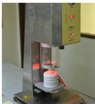
Figure 9. The heat pressing machine. (For2Press® System, bredent UK, Chesterfield, UK)
