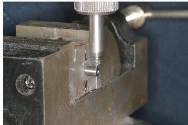
Fig. 2: A model mounted on a lever-type testing machine. Non-impact lateral force of 20N was applied perpendicular to the superstructure, and static strain was recorded for 30 seconds.
