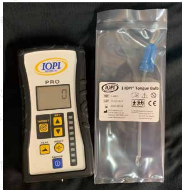
Fig. 2. The Iowa Oral Performance Instruments (IOPI®) Pro and its bulb
