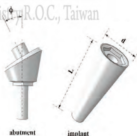
Fig. 2: The implant's design contains three parameters: length (L), diameters (d) and tilt angle (Φ).
