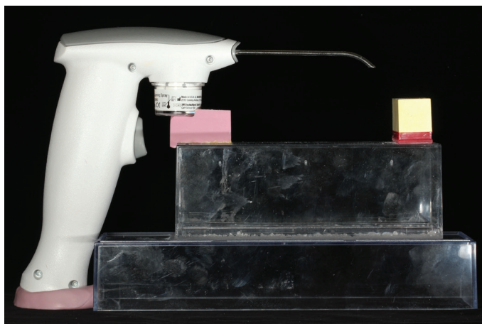
Figure 1. Standardized spraying distance and angle of a powder spraying device
