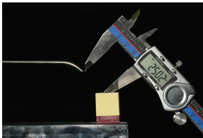
Figure 1. Standardized spraying distance and angle of a powder spraying device
